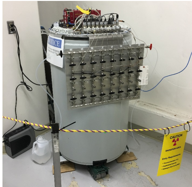
Fig. 10. Gas Generation Shielded Assembly
