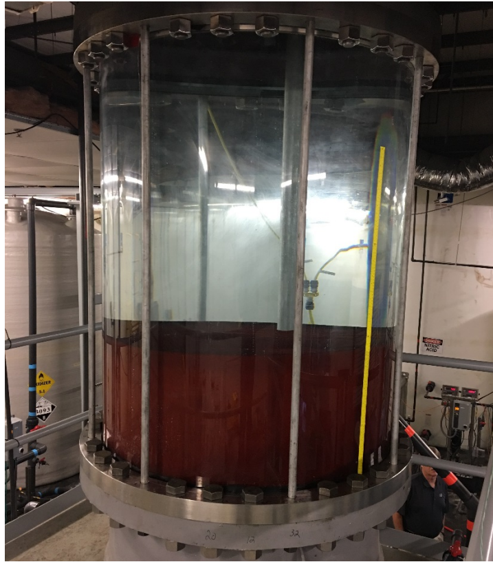
Fig. 13. Full Scale Column with IX Resin
