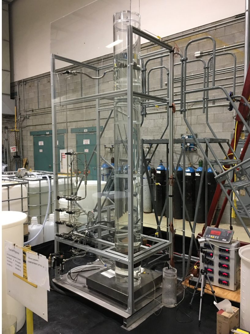
Fig. 11. Gas Retention and Release Assembly
