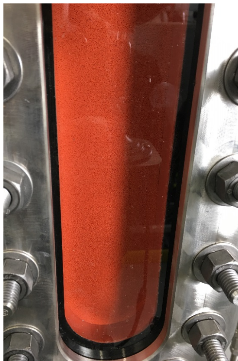
Fig. 8. sRF Resin Loaded in Ion Exchange Column
